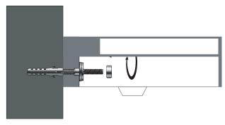
5. Screw a metal nut onto each fixing bolt to secure the basin. Caution: Do not over -tighten, as this may damage the materials.
