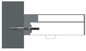
4. Place the basin in position against the wall, iocating the fixing bolts through the holes in the rear of the basin. Push a plastic washer, followed by a metal washer, onto each fixing bolt
