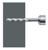
1. Drill two holes in the required position on the wall using a 14mm masonry drill bit, to a depth of 75mm
